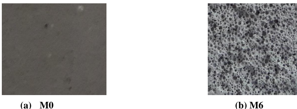
Figure 1: (a & b) The hardened mortar in absence (a) and presense (b) of (CB) after 28 days.
