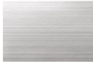
Figure 3. Texture of hairline finishing
