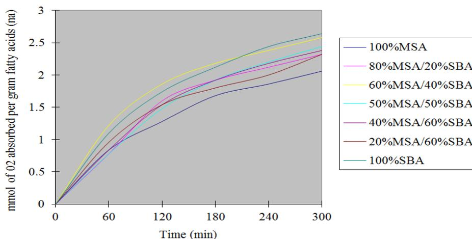
Figure 4. Plots of mmoles/g of Oxygen absorbed (na) vs time for MSA/SBA blends at 60°C
