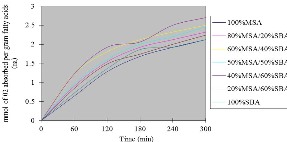
Figure 3. Plots of mmoles/g of Oxygen absorbed (na) vs time for MSA/SBA blends at 45°C
