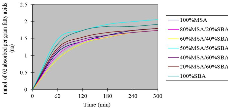
Figure 6. Plots of mmoles/g of Oxygen absorbed (na) vs time for MSA/SBA blends at 90°C
