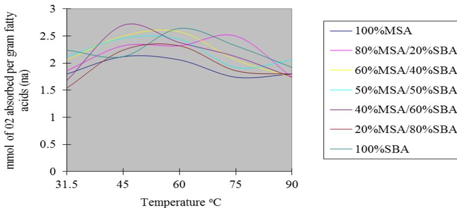
Figure 7. Comparison of 5th-Hour Oxygen absorption of the various blends at 31.5, 45, 60, 75 and 90°C
