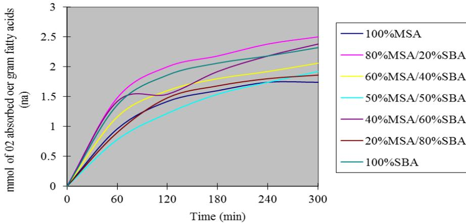
Figure 5. Plots of mmoles/g of Oxygen absorbed (na) vs time for MSA/SBA blends at 75°C
