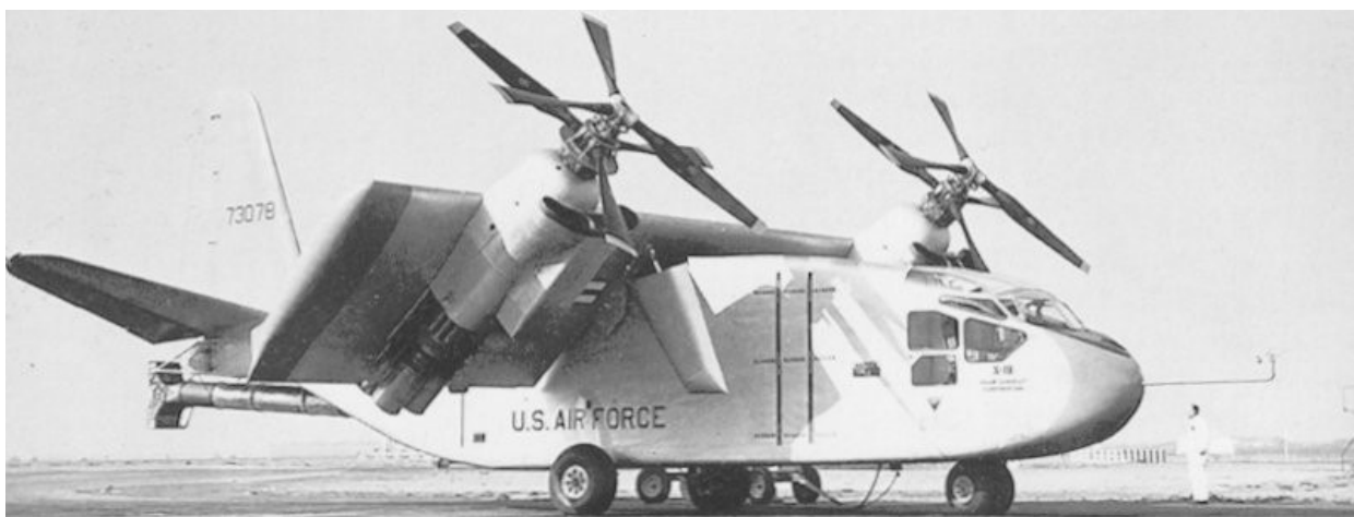
Figure 2. Hiller X-18 uses tilt-wing to perform VTOL manoeuvring.
