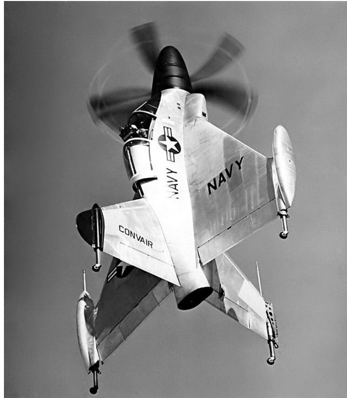
Figure 3. Convair XFY-1 Pogo tail-sitter design.
