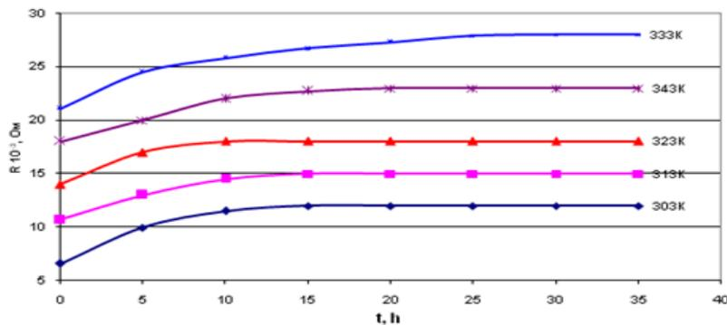
Figure 2. Dependence of electro resistance on duration of corrosion tests for nano-CEC, obtained from electrolyte with concentration  $2 \text{ g/dm}^3\text{C} + 18 \text{ g/dm}^3\text{SiO}_2$
