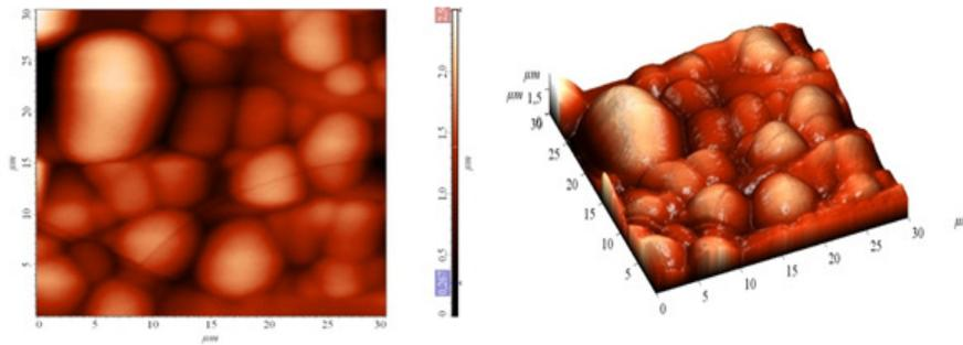
Figure 3. AFM image of nano-CEC Cr-SiO<sub>2</sub>-C, obtained at temperature 303 K
